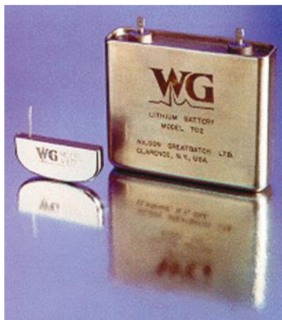
FIGURE 5.16 An early LiI Greatbatch heart pacemaker battery (1972), approximate size 5 \times 8 cm, next to the much smaller 1996 model. (From Wilson Greatbatch Technologies, Inc. With permission.)
