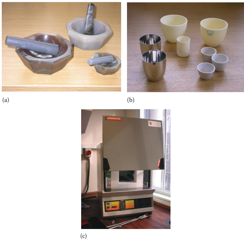
FIGURE 3.1 The basic apparatus for the ceramic method: (a) pestles and mortars for fine grinding; (b) a selection of porcelain, alumina and platinum crucibles; and (c) a furnace.
