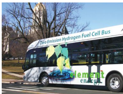
FIGURE 5.19 A zero-emission hybrid fuel cell/ \text{Li}^+ -ion battery-powered bus from UTC Power, operating in Hartford, CT, USA. (From UTC Power. With permission.)
