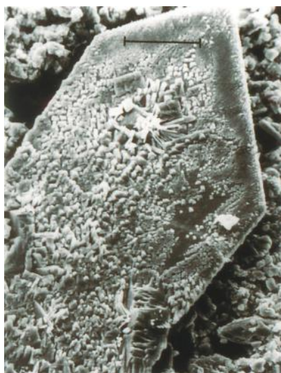
FIGURE 2.17 SEM showing crystals of \text{VSbO}_4 growing out of \beta\text{-Sb}_2\text{O}_4 following reaction with \text{V}_2\text{O}_5 (bar = 40 \mu\text{m} ). (From Professor Berry, F.J., Open University. With permission.)
