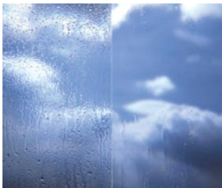
FIGURE 10.25 The difference in performance of ordinary glass and self-cleaning glass. (From Saint Gobain Glass Group.)
